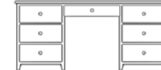
Pencil drawer and 6 equal drawers, 16" wide drawers, 28" knee space 62W x 24D x 30H
